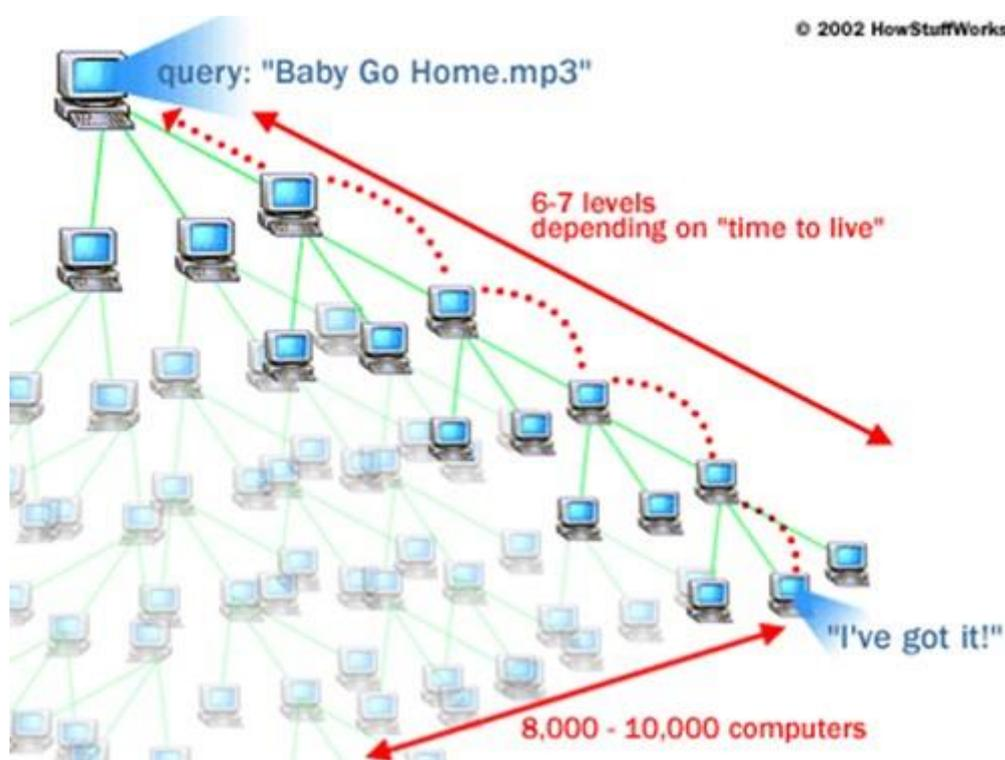
Figure 120: Grokster schematic
